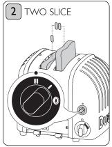
**2 & 4 slot models:** Rotate to the two slice indicator. The first two slots from the left will toast on both sides.
